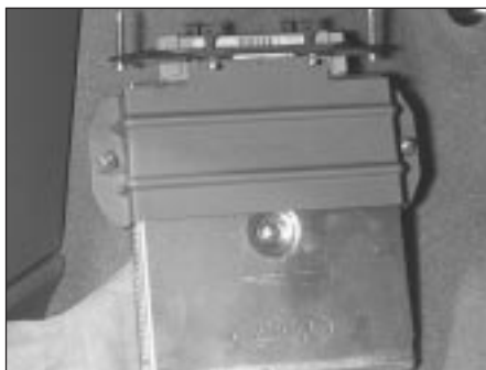
14.37 Withdrawing the EEC IV engine management module into the passenger footwell
