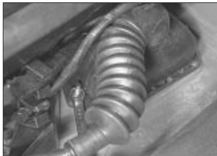
14.36a Undoing the EEC IV engine management module cover retaining nuts (vehicle jack removed for clarity)
